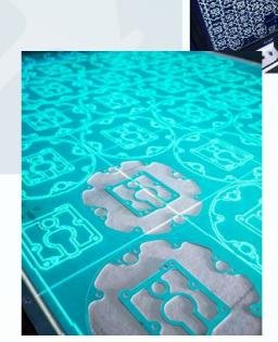
Our Knife Cutting Facility features a robust CNC machine utilising drag or oscillating knife cutting techniques combined with automatic hole punching, for high accuracy conversion of gaskets from sheet material.
