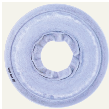
Figure 1: Photos of gasket Material A before testing and after testing at a surface pressure of 160 N/mm 2
