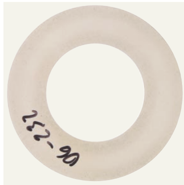
Figure 4: Photos of gasket KLINGER®top-chem 2003 before and after the P_{QR} -test.
