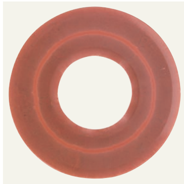
Figure 9: Photos of gasket KLINGER®top-chem 2005 before testing and after testing at a surface pressure of 60 N/mm 2
