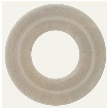
Figure 7: Photos of gasket KLINGER®top-chem 2000 before testing and after testing at a surface pressure of 160 N/mm 2
