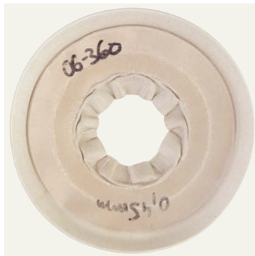
Figure 3: Photos of gasket KLINGER®top-chem 2003 before testing and after testing at a surface pressure of 200 N/mm 2
