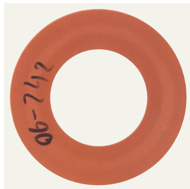
Figure 10: Photos of gasket KLINGER®top-chem 2005 before and after the P_{QR} -test
