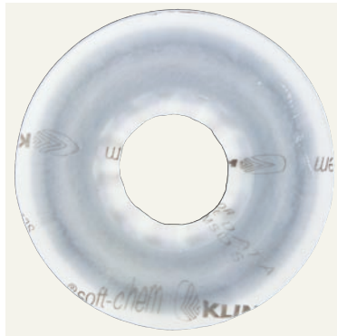
Figure 5: Photos of gasket KLINGER®soft-chem before testing and after testing at a surface pressure of 200 N/mm 2
